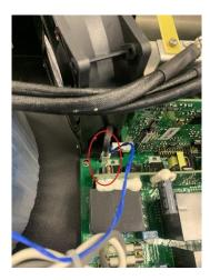
5. Mount the SPR00090 fan PWM converter PCBA (with the short wires) with the supplied tie-wraps to the mounting eyes/holes of the fan. Connect the wire of the fan to the connection on the new fan control PCBA. Plug the connector of the new PWM converter PCBA to the original fan connector on the main board, as shown on the pictures below.
